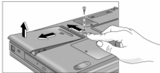
Figure 2-4. Removing the Hard Disk Drive
